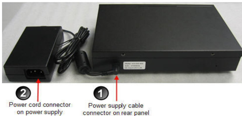
Figure 23 Attaching the power cables on the ET0010A-402
